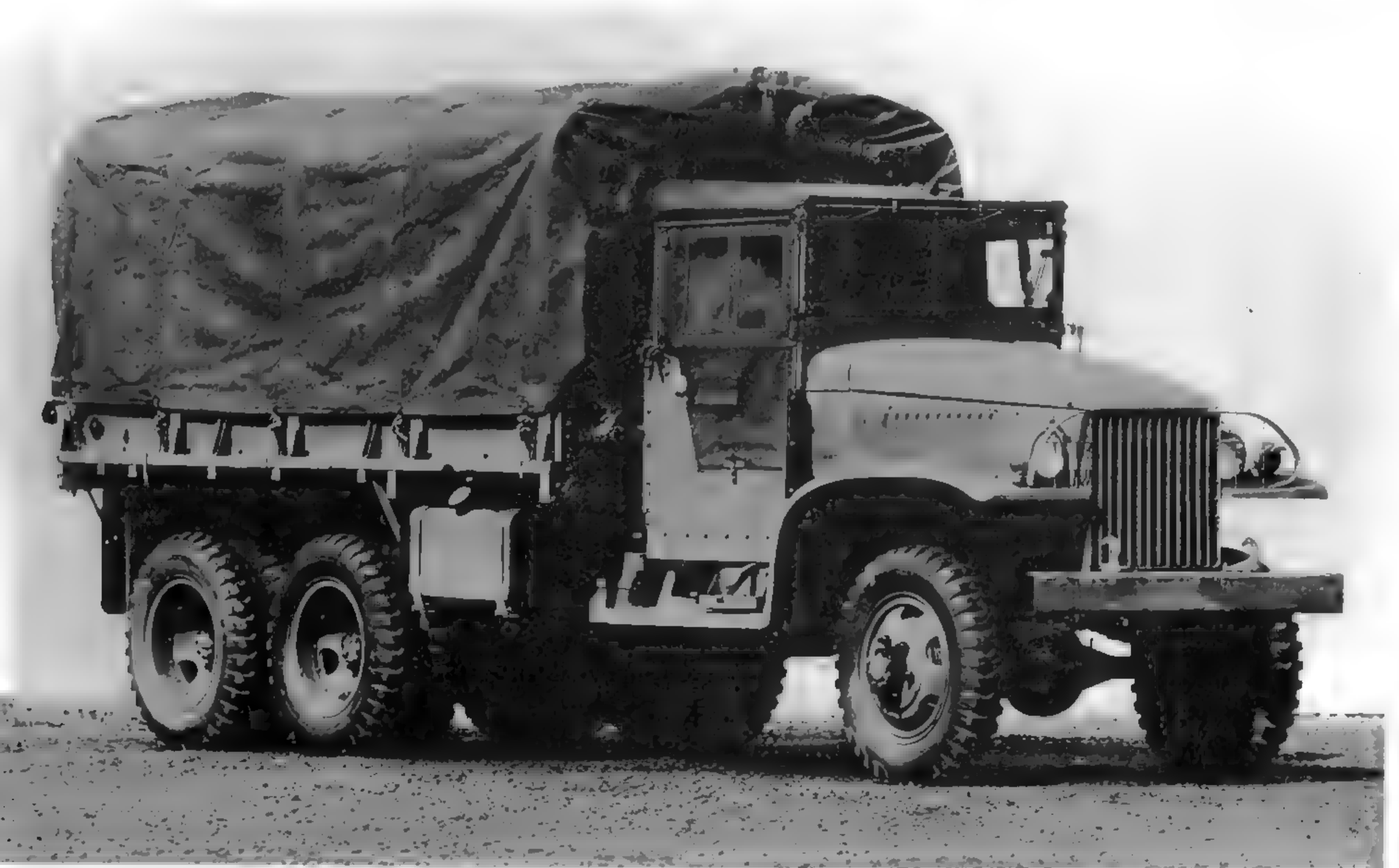
Frames were different for trucks that were winch not equipped, and so was the size of the front bumper. (U.S. Army photo)
